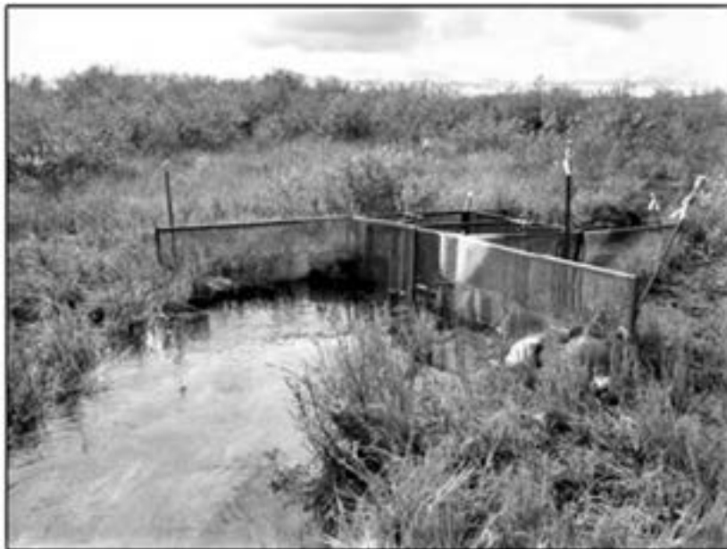
Figure 2-6 Upstream/downstream fish trap box 2 installed June 9, 2015 on the Pigeon Stream, Ekati. (ERM, 2016) Data obtained from this trap were used for comparison to the cameras.
