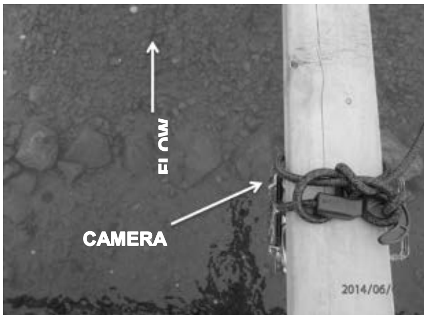
Figure 2-15 Top of Camera #1 mounted on the South side of the downstream bridge over the PSD in 2014 (photo by author).
