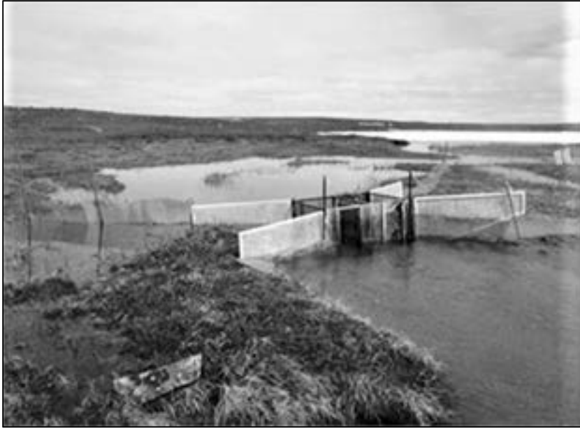
Figure 2-7 Upstream/downstream fish trap box 3 installed early June, 2014 on the Pigeon Stream, Ekati. (ERM, 2015) Data obtained from this trap were used for comparison to the cameras.
